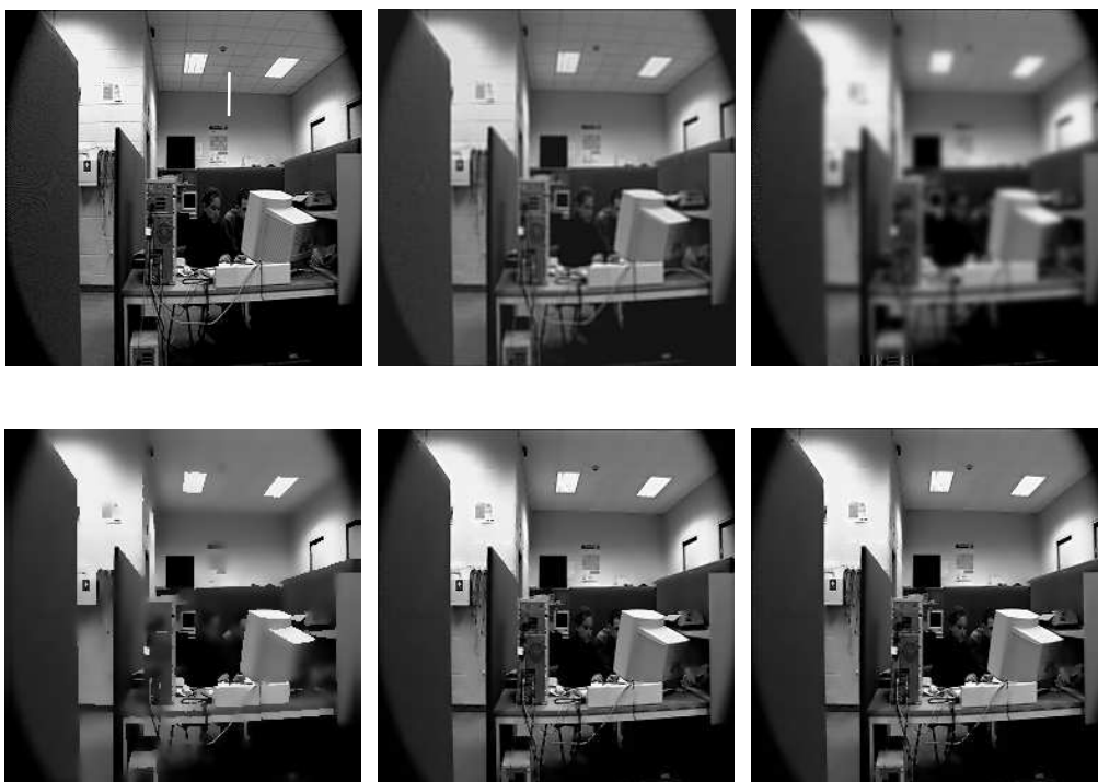
Figure 1: Results from each of the smoothing filters, top-row, l-to-r is the original image, image after Savitzky-Golay and Gaussian. Bottom-row, Adaptive, Nonlinear Diffusion and Anisotropic Gaussian.
